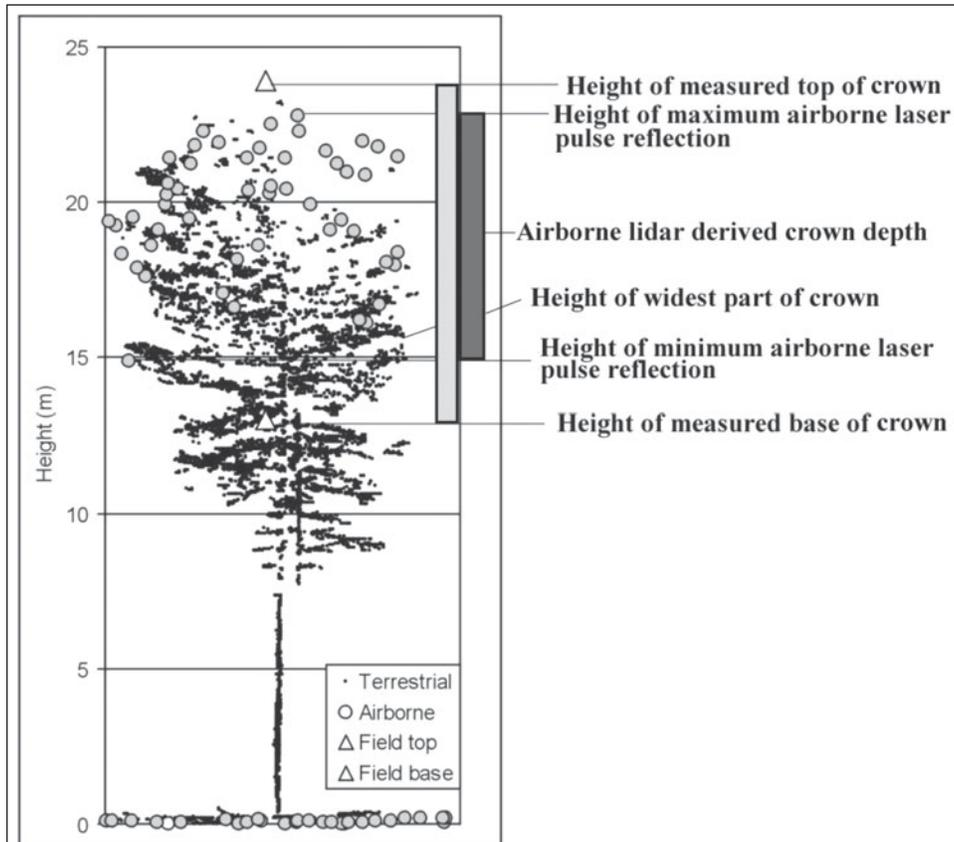
**Figure 4.** Airborne and terrestrial lidar point cloud data for a sample tree, illustrating differences between maximum and minimum laser pulse returns within the crown (in comparison with measured top-of-live-crown and base-of-live-crown). Depth-of-crown between maximum and minimum laser pulse returns is significantly underestimated compared with field measurements.
